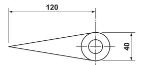
Add the minute hand to the clock face in a vertical position to a scale of 1:2.
